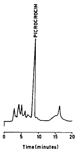
Fig. 2. HPLC profile of picrocrocine. Solvent, gradient run from 20 to 80% (v/v) acetonitrile in water in 20 min; flow-rate, 0.5 ml/min; column, Shimadzu CLC-ODS (150 mm × 4.9 mm I.D.); detection wavelength, 250.5 nm.
